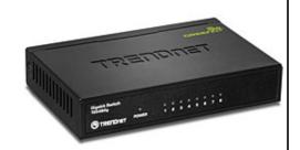
The compact 8-Port Gigabit GREENnet Switch provides high bandwidth performance, ease of use and reliability, all while reducing power consumption by up to 70%. GREENnet technology automatically adjusts power voltage as needed, resulting in substantial energy savings.
