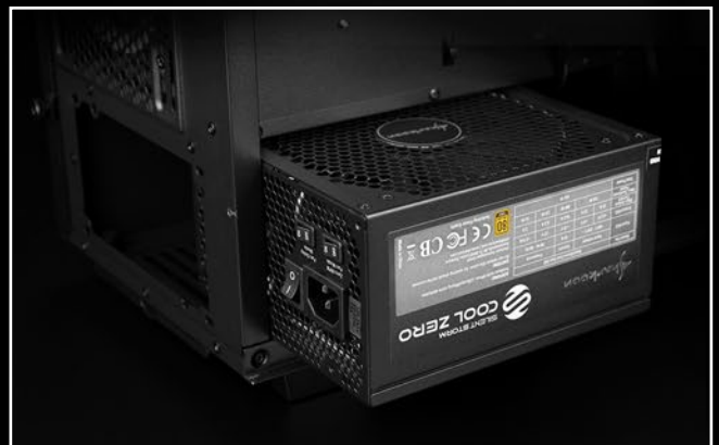
Power Supply Fan Installed Upwards
