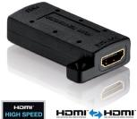
Passive HDMI cable can transmit a 1080p signal up to 15 meters only. From that length the signal loss is too large, the result is "digital snow" Interference or completely blank screens. The PureLink HDMI repeater PI090 is an intelligent HDMI amplifier and increases the maximum cable length between the video source and video sink in full HDTV resolution up to 35m.
