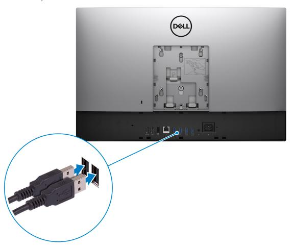
${\bf 3.}\;$  Connect to your network using a cable, or connect to a wireless network.
