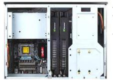
Although the chassis measures only 325mm deep, it can support powerful graphics cards for high end configurations.
