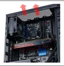
Supports 120mm radiator in the rear; Enlarged top vents
