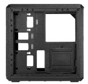
**Clean routing space** 28mm of space behind the motherboard tray allow for easy and hidden cable management.
