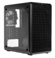
**Tempered glass side panel** Show off your build through the 4mm-thick tempered glass side panel, easily installed with thumbscrews.
