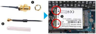
8. Install the antenna cable connectors through the appropriate opening at the back of the chassis. When leading the cable connector through the opening, check the socket alignment and only push horizontally. DO NOT turn or twist the cable. Should any difficulties occur, make sure the surface is clean. Finally, check the alignment again and carefully apply more force.
