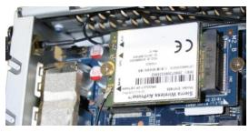
The installed riser card with additional LTE/4G card (top view) and SIM card (hidden). The pre-installed WLAN card and WLAN antenna must be removed before.
