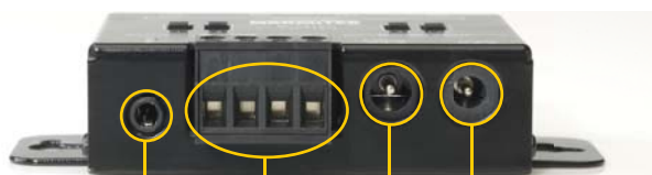
IR INPUT: Single Receiver IR INPUT: Multiple Receivers (up to 6) POWER INPUT: Status adapter POWER INPUT: Power adapter
