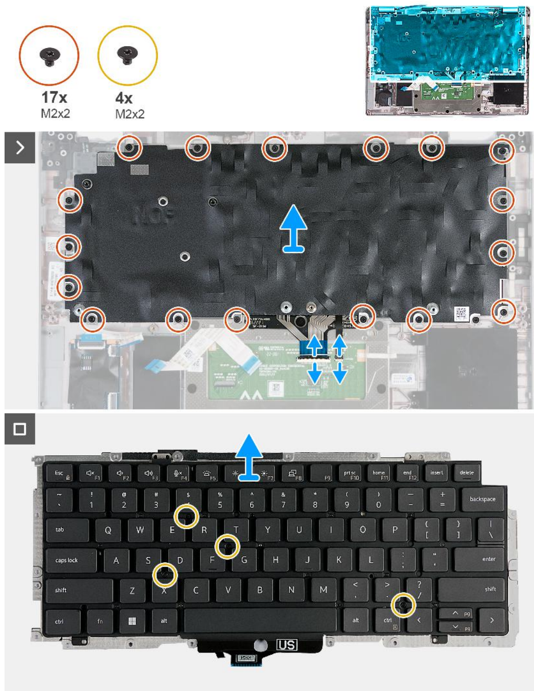
Figure 61. Removing the keyboard
