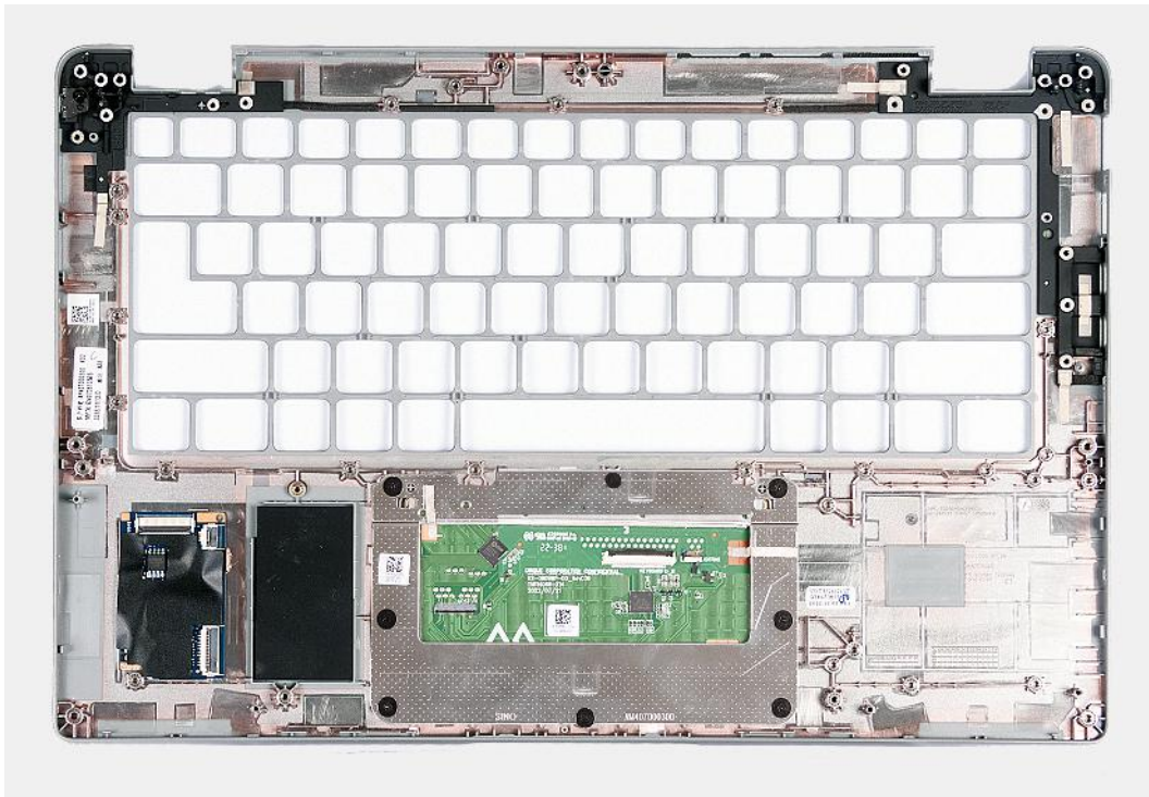
Figure 64. Installing the palm-rest assembly
