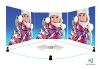
IPS displays use an advanced technology which gives you extra wide viewing angles of 178/178 degree, making it possible to view the display from almost any angle - even in 90 degree Pivot mode! Unlike standard TN panels, IPS displays gives you remarkably crisp images with vivid colors, making it ideal not only for Photos,
