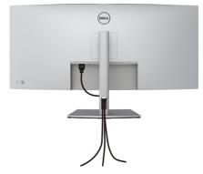
After attaching all necessary cables to your monitor and computer, (see **Connecting Your Monitor** for cable attachment) organize all cables as shown above.
