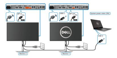
Similarly, a PC is connected to two monitors in an initially ON power state, and the PC system power state is in sync with Monitor 1 power button. When you press Monitor 1 or PC power button, both Monitor 1 and PC are turned OFF, Meanwhile. Monitor 2 remains in Standby mode. You need to manually press the power button on Monitor 2 to turn it OFF.
