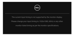
This means that the monitor cannot synchronize with the signal that it is receiving from the computer. See Monitor specifications for the Horizontal and Vertical frequency ranges addressable by this monitor. Recommended mode is  $1920 \times 1080$ .
