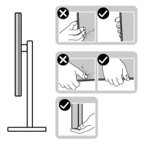
When lifting or moving the monitor, ensure the screen is facing away from you and do not press on the display area to avoid any scratches or damage.
