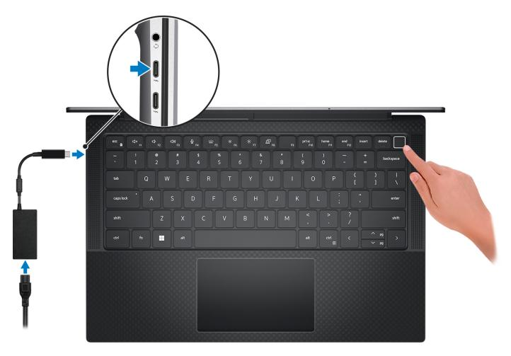
**NOTE:** To conserve battery power, the battery might enter power saving mode. Connect the power adapter and press the power button to turn on the computer.
