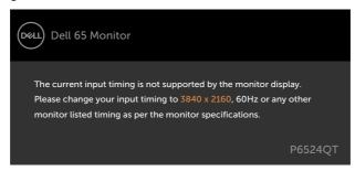
This means that the display cannot synchronize with the signal that it is receiving from the computer. See Display Specifications for the Horizontal and Vertical frequency ranges addressable by this display. Recommended mode is  $3840 \times 2160$ .
