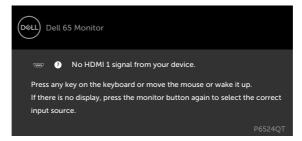
If either HDMI 1, HDMI 2, HDMI 3, DP or USB Type-C input is selected and the corresponding cable is not connected, a floating dialog box as shown below appears.
