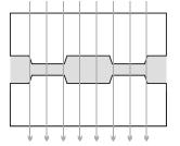
Since air isknown as a poor heat conductor, it should be replaced by a more conductive material to improve heat flow across thermal interfaces.
