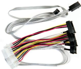
The Adaptec I-HDmSAS-4SAS-SB-.8M is an internal Mini-SAS HD x4 (SFF-8643) to (4) x1 Serial Attached SCSI (SFF-8482 adapter based) fan-out cable with sideband signals. It measures 0.8 meters and is used for connecting a Series 7/7Q adapter to SAS disks.
