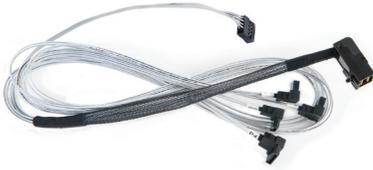
The Adaptec I-rA-HDmSAS-4rASATA-SB-.8M is an internal “right angle” Mini-SAS HD x4 (SFF-8643) to “right angle” (4) x1 Serial ATA fan-out cable with sideband signals. It measures 0.8 meters and is used for connecting a Series 7/7Q adapter to SATA disks, or a SAS/SATA backplane.
