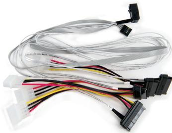
The Adaptec I-rA-HDmSAS-4SAS-SB-.8M is an internal “right angle” Mini-SAS HD x4 (SFF-8643) (4) x1 Serial Attached SCSI (SFF-8482, adapter based) fan-out cable with sideband signals. It measures 0.8 meters and is used for connecting a Series 7/7Q adapter to SAS disks.
