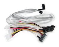
The Adaptec I-rA-HDmSAS-4SAS-SB-.8M is an internal "right angle" Mini-SAS HD x4 (SFF-8643) (4) x1 Serial Attached SCSI (SFF-8482, adapter based) fan-out cable with sideband signals. It measures 0.8 meters and is used for connecting a Series 7/7Q adapter to SAS disks.
