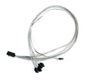
The Adaptec I-HDmSAS-4SATA-SB-.8M is an internal Mini-SAS HD x4 (SFF-8643) to (4) x1 Serial ATA (adapter based) fan-out cable with sideband signals. It measures 0.8 meters and is used for connecting a Series 7/7Q adapter to SATA disks, or a SAS/SATA backplane.
