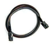
The Adaptec I-HDmSAS-mSAS-1M is an internal Mini-SAS HD x4 (SFF-8643) to Mini-SAS (SFF-8087) x 4 cable. It measures 1 meter and is used for connecting a Series 7/70 adapter to a SAS/SATA backplane.
