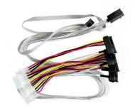
The Adaptec I-HDmSAS-4SAS-SB-.8M is an internal Mini-SAS HD x4 (SFF-8643) to (4) x1 Serial Attached SCSI (SFF-8482 adapter based) fan-out cable with sideband signals. It measures 0.8 meters and is used for connecting a Series 7/7Q adapter to SAS disks.
