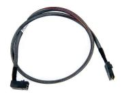
The Adaptec I-rA-HDmSAS-mSAS-.8M is an internal "right angle" Mini-SAS HD x4 (SFF-8643) to Mini-SAS (SFF-8087) x4 cable. It measures 0.8 meters and is used for connecting a Series 7/7Q adapter to a SAS/SATA backplane.
