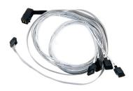
The Adaptec I-rA-HDmSAS-4SATA-SB-.8M is an internal "right angle" Mini-SAS HD x4 (SFF-8643) to (4) x1 Serial ATA (adapter based) fan-out cable with sideband signals. It measures 0.8 meters and is used for connecting a Series 7/7Q adapter to SATA disks, or a SAS/SATA backplane.
